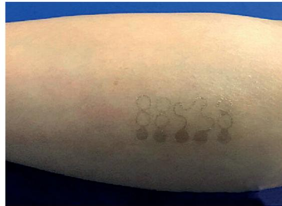
Fig. 2. Tech-tattoo made with one-atom size, two-dimensional single layer of graphene. Contrary to regular temporary tattoos, graphene tattoo is almost transparent. Image credit: Shideh Kabiri Ameri, Deji Akinwande, et al.
